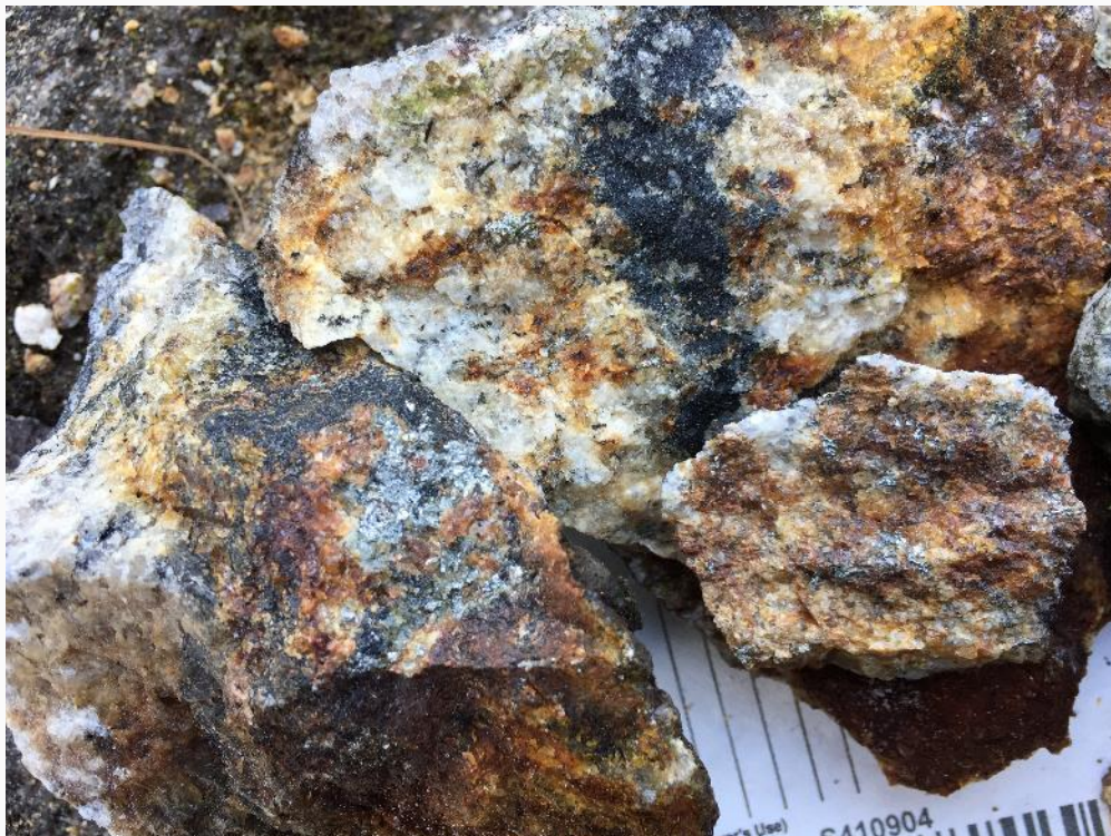
S410904 (float) Tonalite with disseminated arsenopyrite and quartz-tourmaline veinlets (same float as S410905) 1.1 g/t Au
