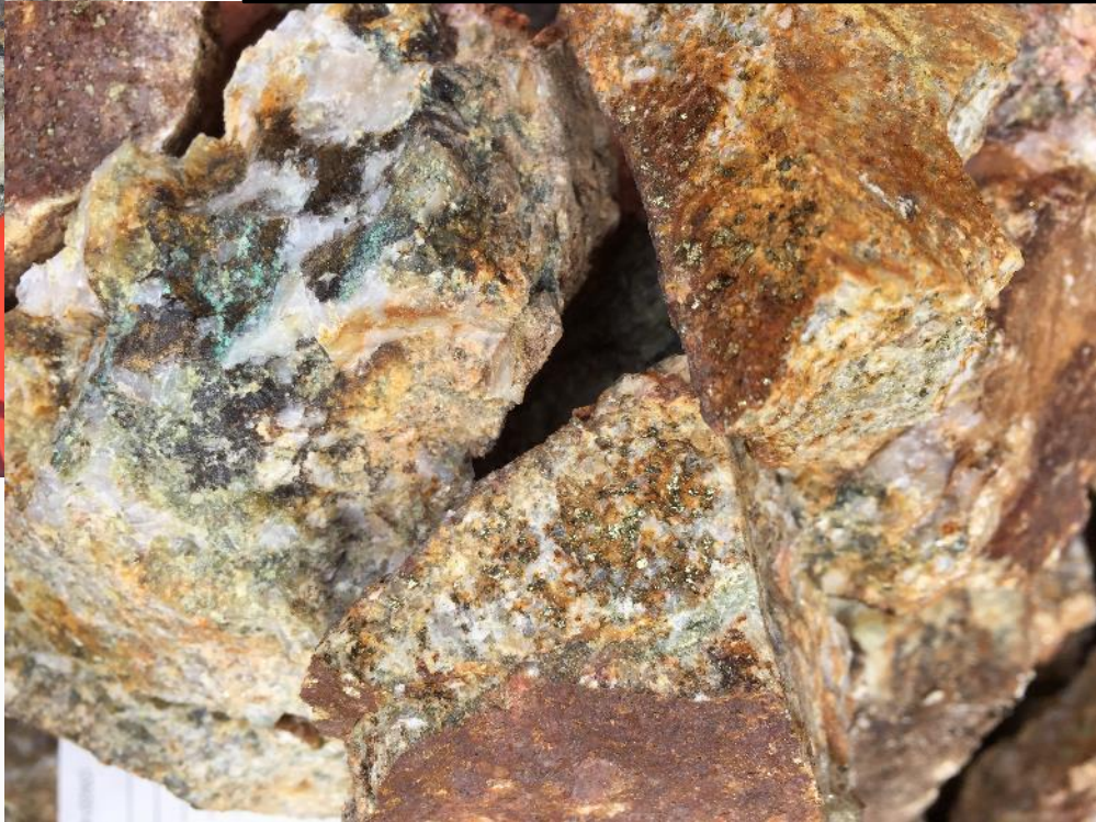
S410738 (outcrop) Granite, altered in chlorite-epidote, injected with quartz and ankerite veins 0.34 % Cu, 0.02 % Mo
