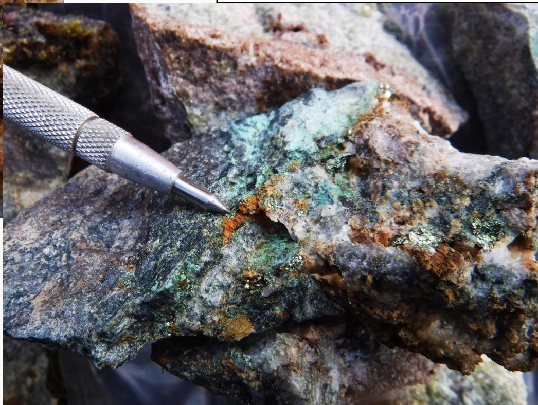
S410629 (float) Strongly chloritized granite with intense quartz-chlorite stockwork, vein and disseminated chalcopyrite+malachite 0.26 % Cu
