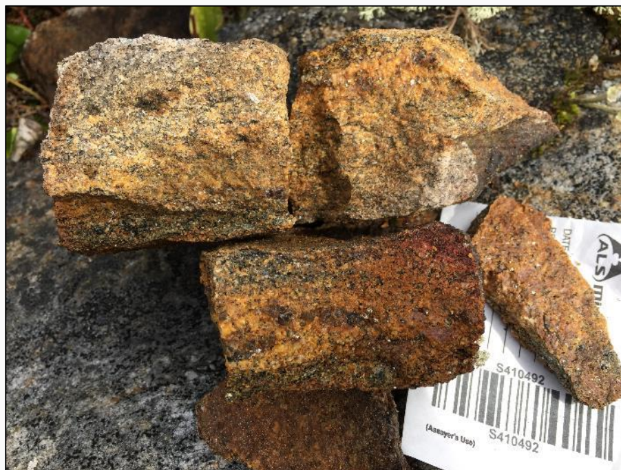
S410492 (float) Granodiorite with granite dykes, quartz veinlets, biotite alteration and 1% pyrite 2.84 g/t Au, 0.06 % Cu, 2.0 g/t Ag
