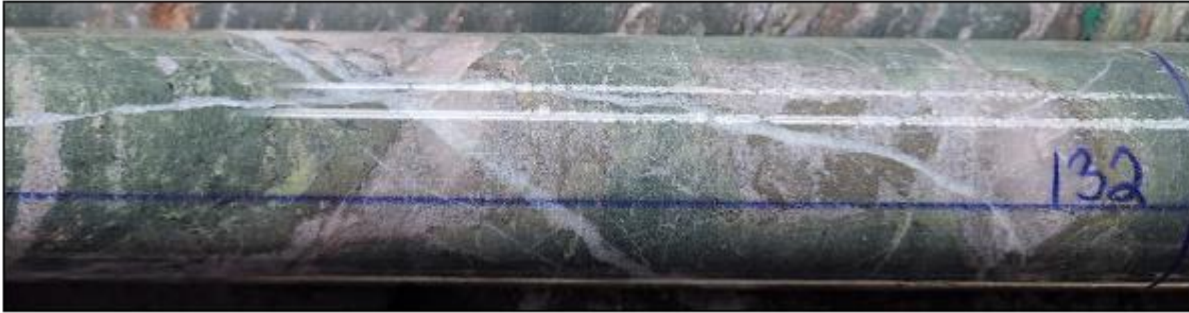
Figure 6: Silicified V3B with quartz veining and disseminated and patchy Py mineralization.
