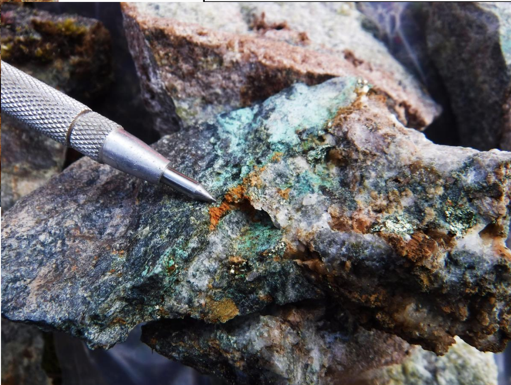
S410629 (float) Strongly chloritized granite with intense quartz-chlorite stockwork, vein and disseminated chalcopyrite+malachite 0.26 % Cu
