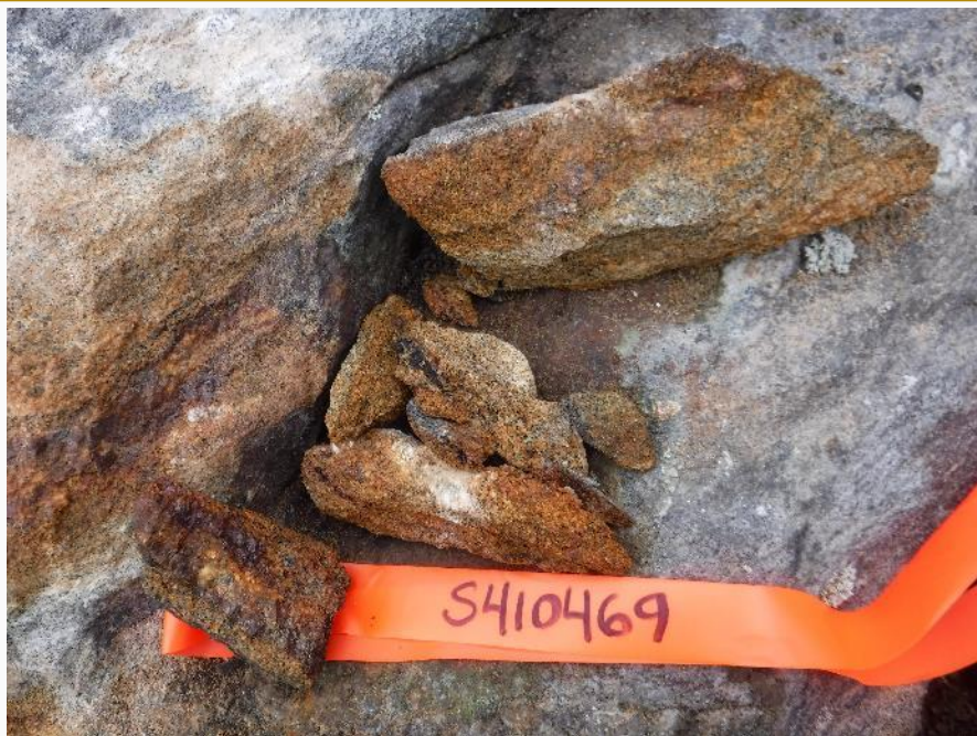
S410469 (float) Granodiorite with bands altered in biotite and mineralized in trace magnetite and chalcopyrite 2.83 g/t Au, 0.13 % Cu, 15.2 g/t Ag
