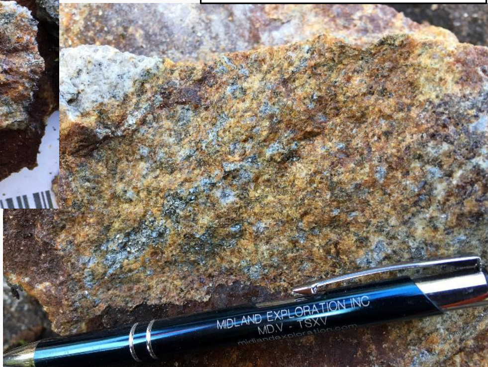
S410905 (float) Sheared tonalite with disseminated arsenopyrite, quartz-tourmaline veinlets, quartz veinlets 3.47 g/t Au
