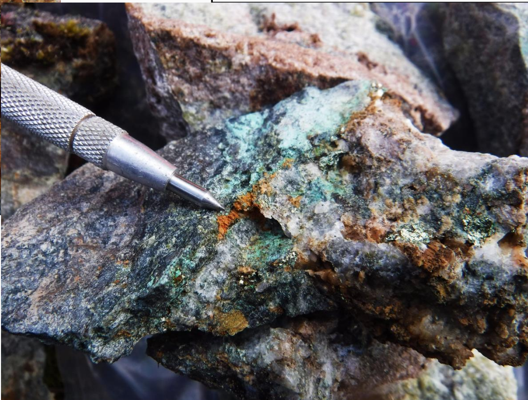
S410629 (float) Strongly chloritized granite with intense quartz-chlorite stockwork, vein and disseminated chalcopryite+malachite 0.26 % Cu
