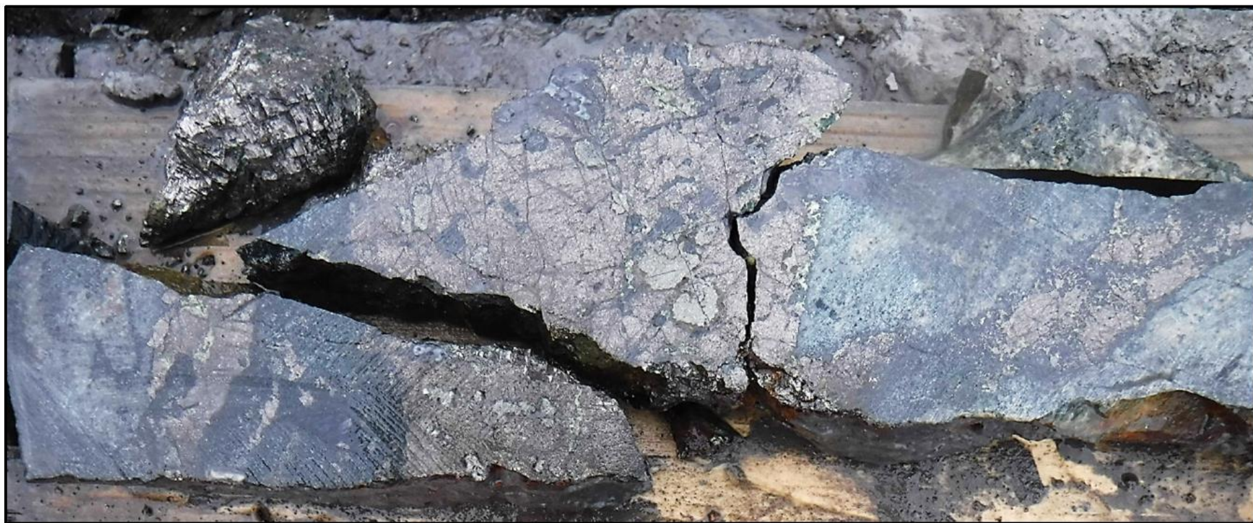
Figure 26: Example of massive mineralization encountered in Papavoine channels. Massive pyrrhotite with clusters of chalcopyrite inside (sample X915634 from PPV-18-04).
