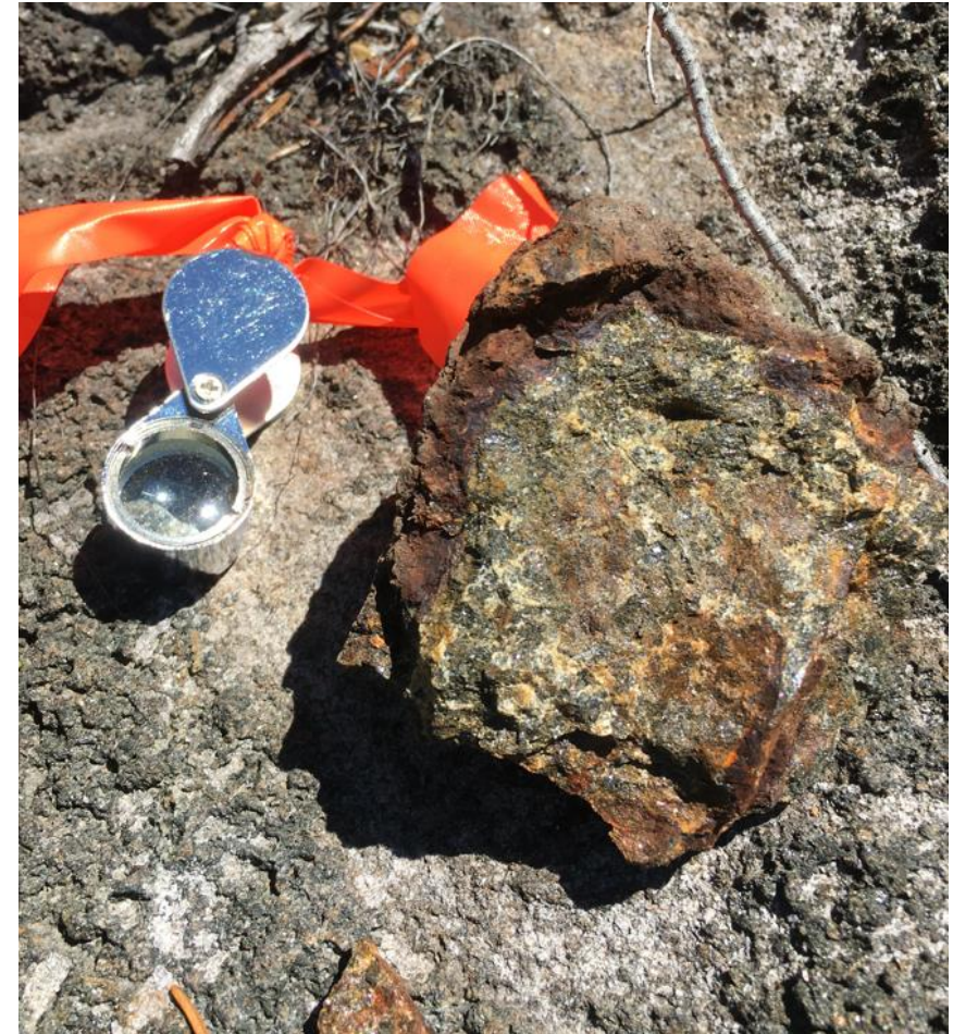
Anomalous Ni-Cu with high Tenor at 100% Sulfides (5% Ni)
