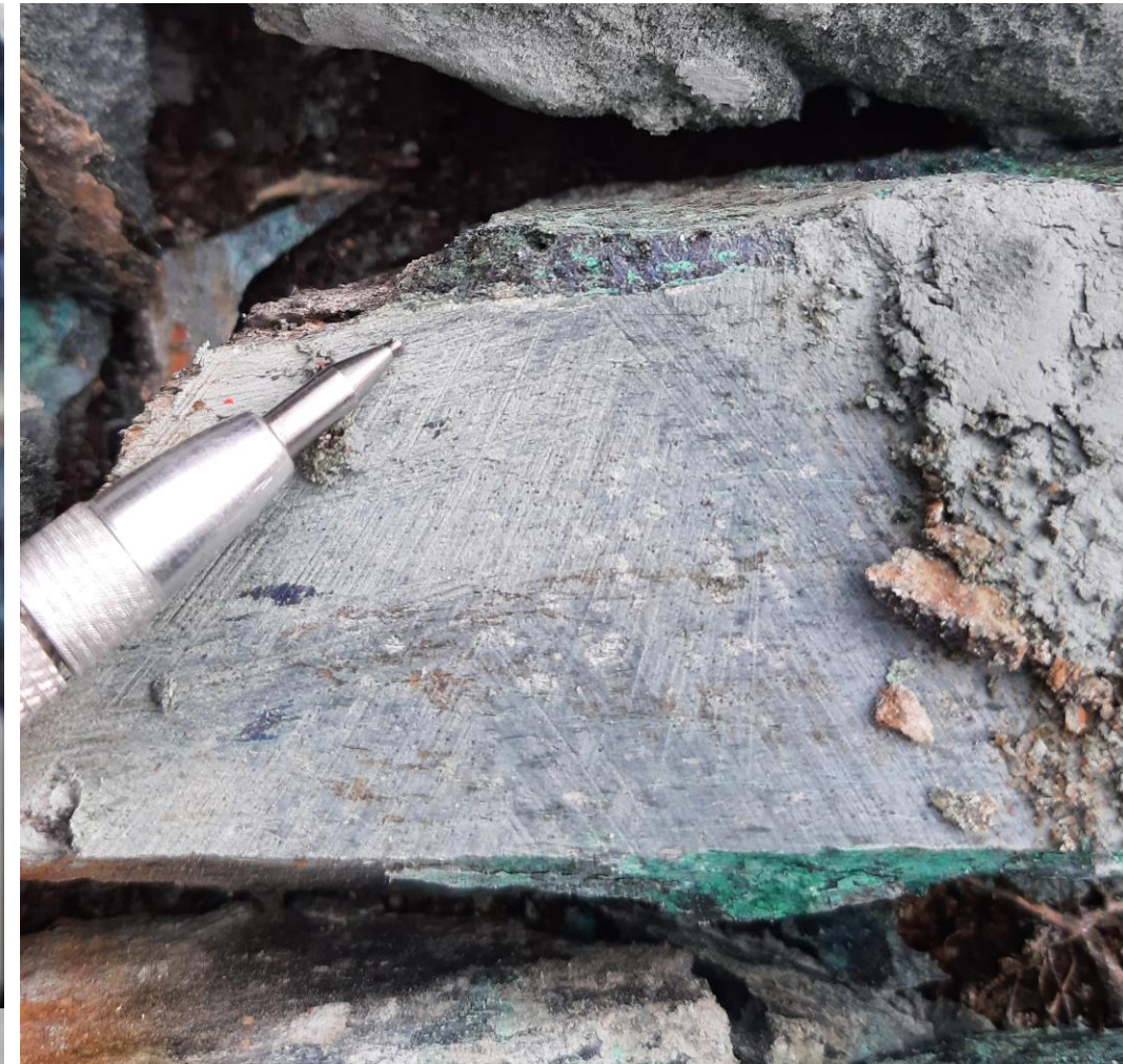
(c) channel 2, #C879224 : 1.17 % Cu, 0.56 g/t Au, 8.8 g/t Ag over 0.5 metres
