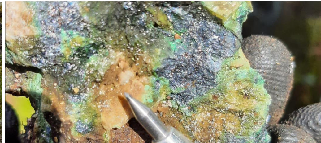
(b) #C879209 – carbonate and bornite, malachite vein 25.60 % Cu, 4.90 g/t Au, 162.0 g/t Ag
