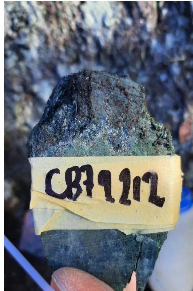
(b) channel 1, #C879212 : 3.56 % Cu, 1.55 g/t Au, 25.0 g/t Ag over 0.5 metres
