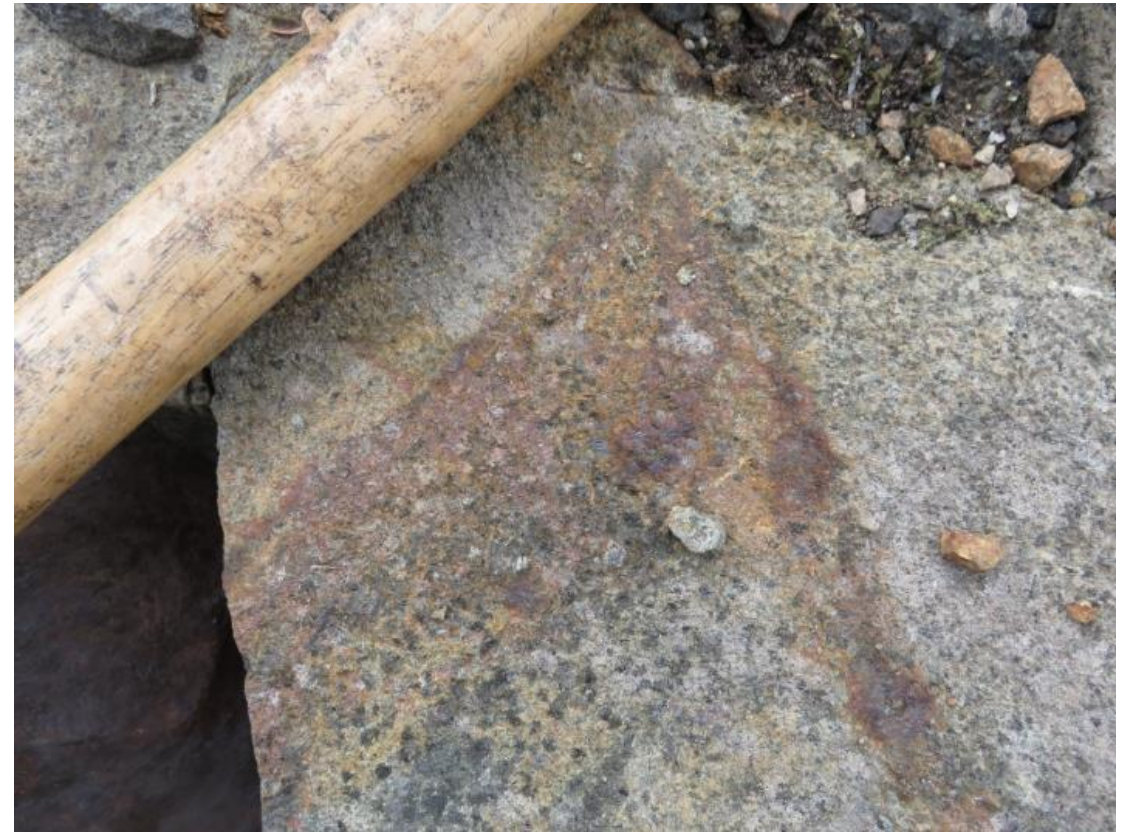
Magmatic breccia. Pyroxenite to melagabbonorite matrix with heavily disseminated sulfides. Clasts are all autoliths
