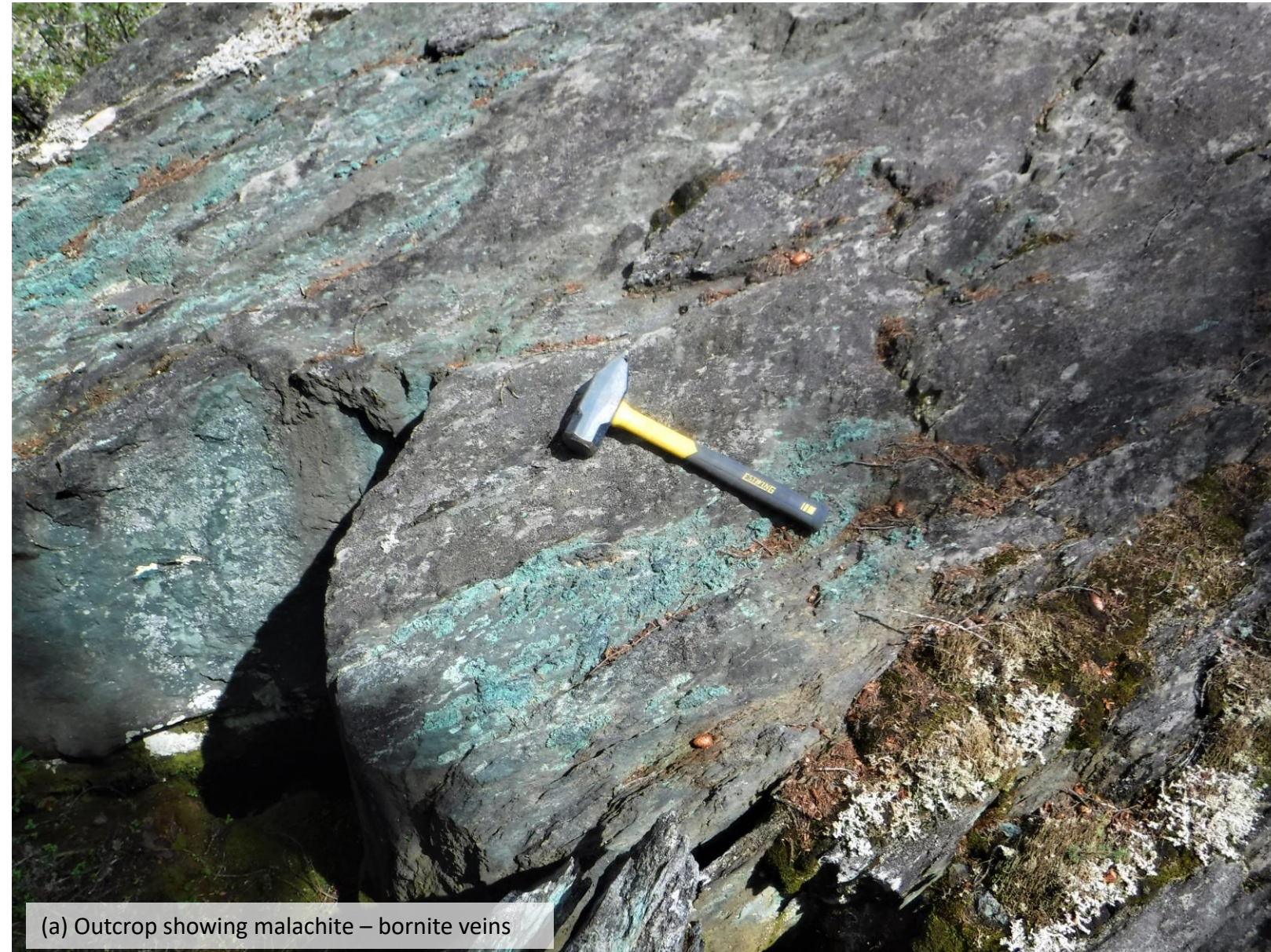
(b) malachite – bornite veins at surface
