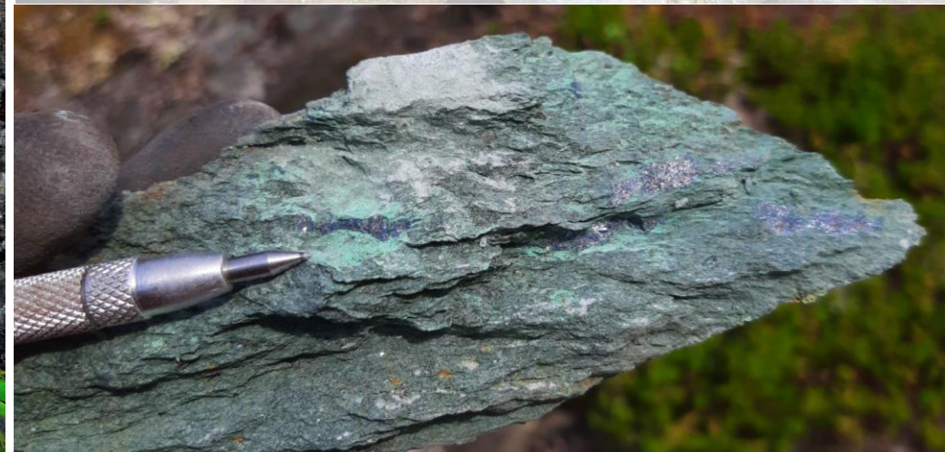
(c) #C878500 – 3% malachite and bornite mineralization in a mafic schist
