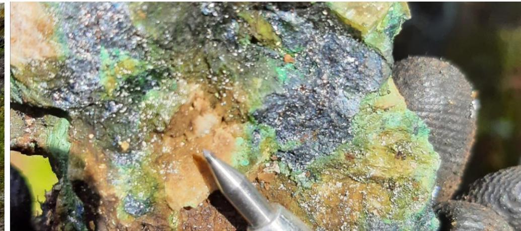
(b) #C879209 – carbonate and bornite, veine de malachite
