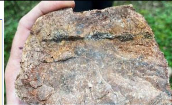
Massive py veinlet in silicified intermediate dyke
