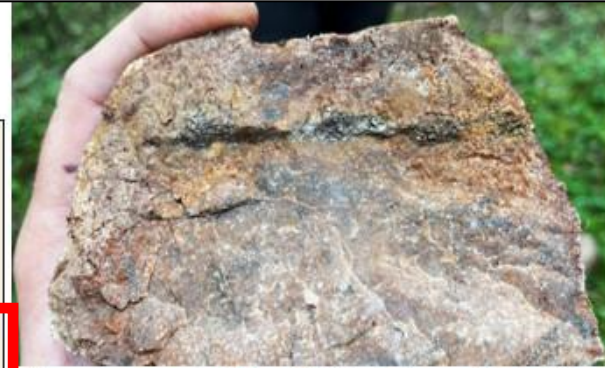
Massive py veinlet in silicified intermediate dyke
