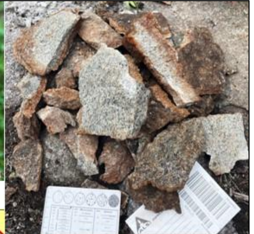
Close up of cb-chl alteration in bt-rich intermediate dyke
