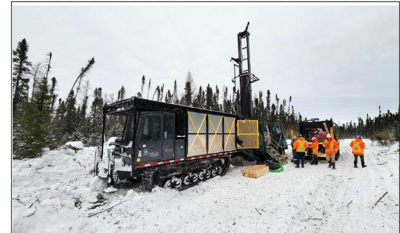
Figure 1: Wallbridge Geologists visiting Earth Drilling's LS600 sonic drill during the February 2023 sonic program.
