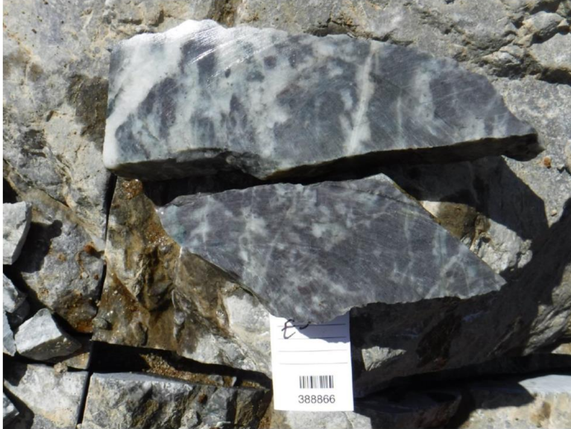
Figure 17: EJV2018TR007-R1; Intense silicification and hydrothermal breccia over 3 meters.
