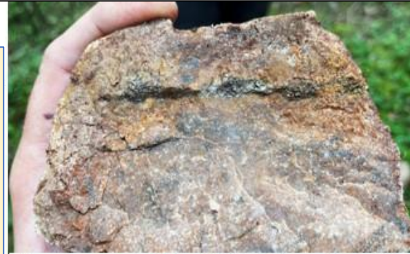
Massive py veinlet in silicified intermediate dyke
