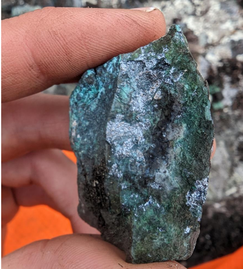
39.90 % Cu, 308.00 g/t Ag, 0.04 g/t Au Massive bornite, digenite, malachite in a dm-scale calcite vein (#C1456513 )
