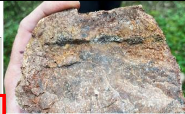
Massive py veinlet in silicified intermediate dyke
