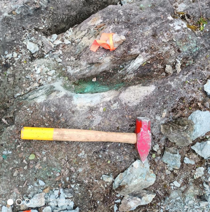
5.98 %Cu, 22.00 g/t Ag, 0.08 g/t Au Fracture-filling malachite-digenite mineralization (#C1456166 )
