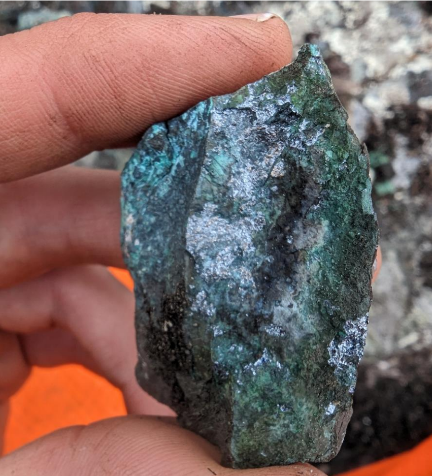
39.90% Cu, 308.0 g/t Ag, 0.04 g/t Au Massive bornite, digenite, malachite in a dm-scale calcite vein (#C1456513 )
