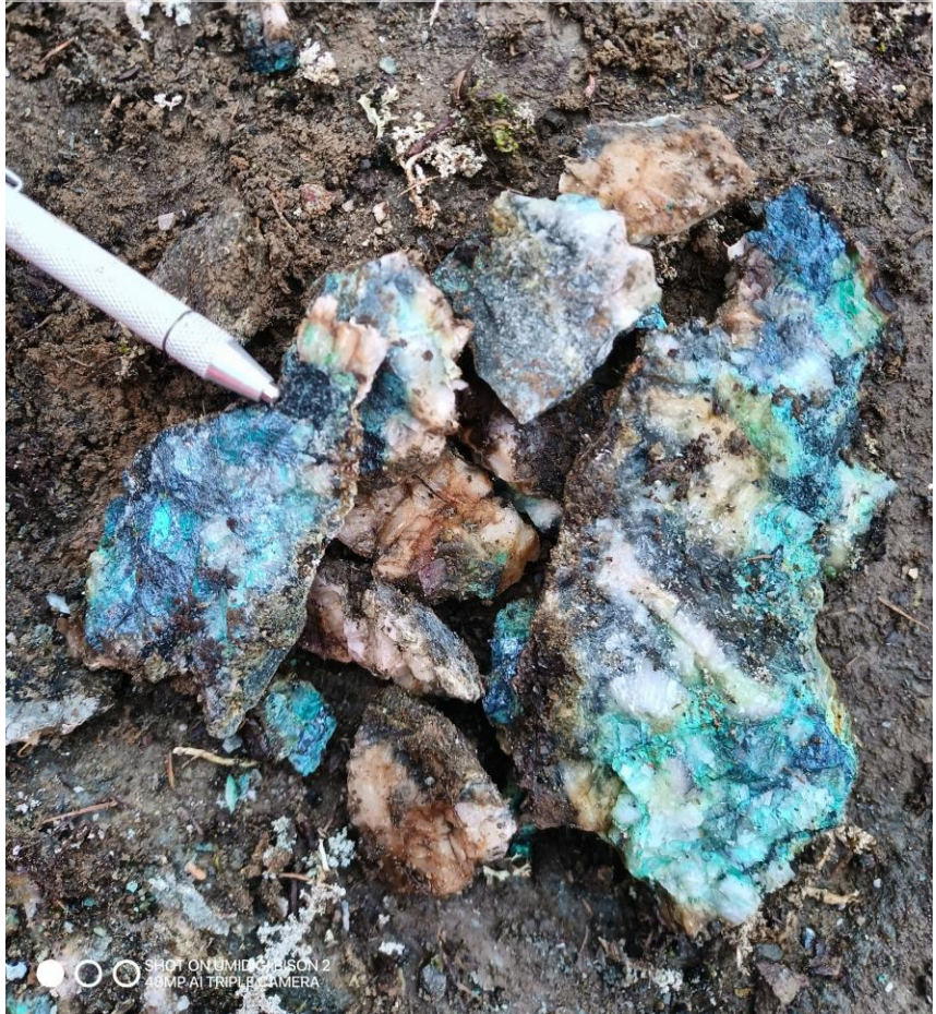
23.90 % Cu, 238.0 g/t Ag, 1.40 g/t Au Digenite, malachite, bornite, calcite vein, cm scale (#C1456119)
