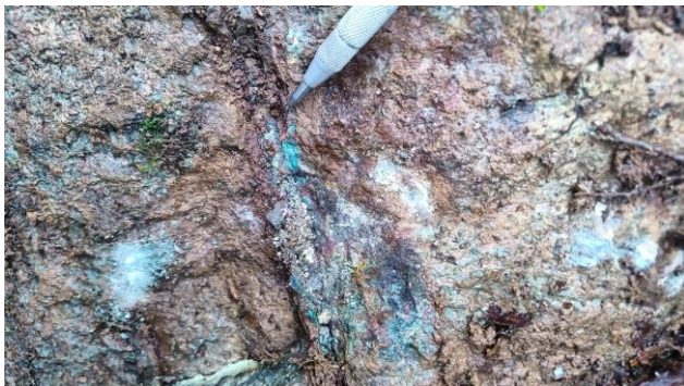
< C1456034 : 0.47% Cu, 57 ppm Co Outcrop of epidotized and hematized gabbro, affected by fractures and calcite veinlets containing 2% chalcopyrite and malachite and in a halo
