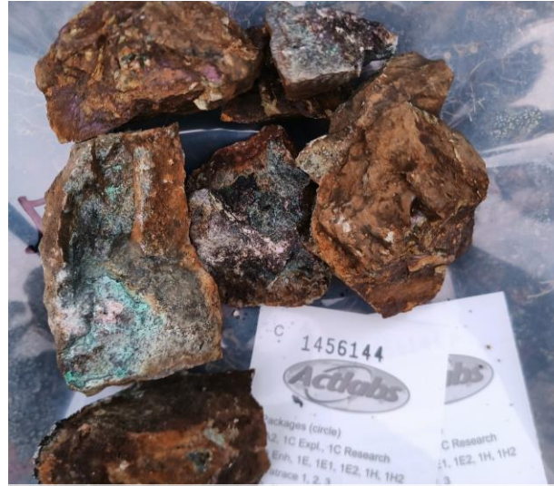
C1456144 : 0.54% Cu, 41 ppm Co Epidotized gabbro outcrop containing 7% cm malachite and 3% chalcopyrite
