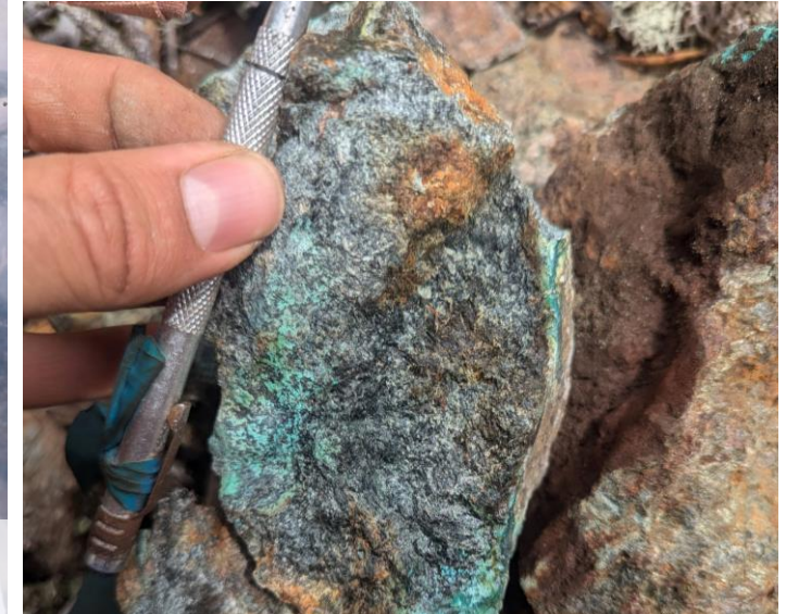
C1456534 : 1.94% Cu, 143 ppm Co, 52 ppb Au, 18 ppm Mo Gabbro affected by chalcopyrite (5%) and pyrite (2%) veinlets with potassic alteration and associated albitization
