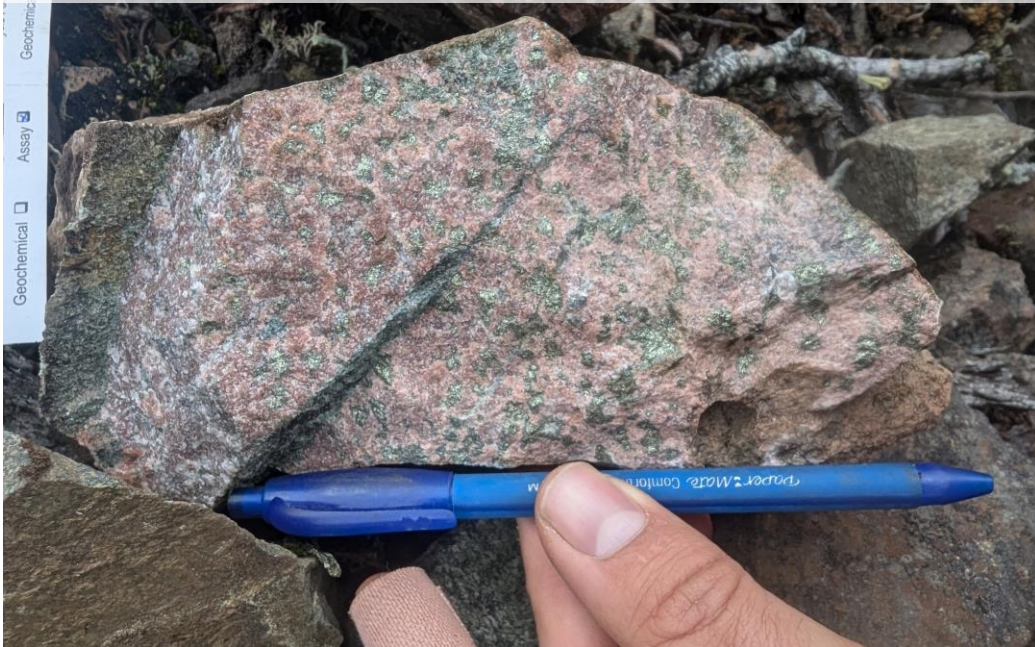
< C1456034 : 0.47% Cu, 57 ppm Co Outcrop of epidotized and hematized gabbro, affected by fractures and calcite veinlets containing 2% chalcopyrite and malachite and in a halo
