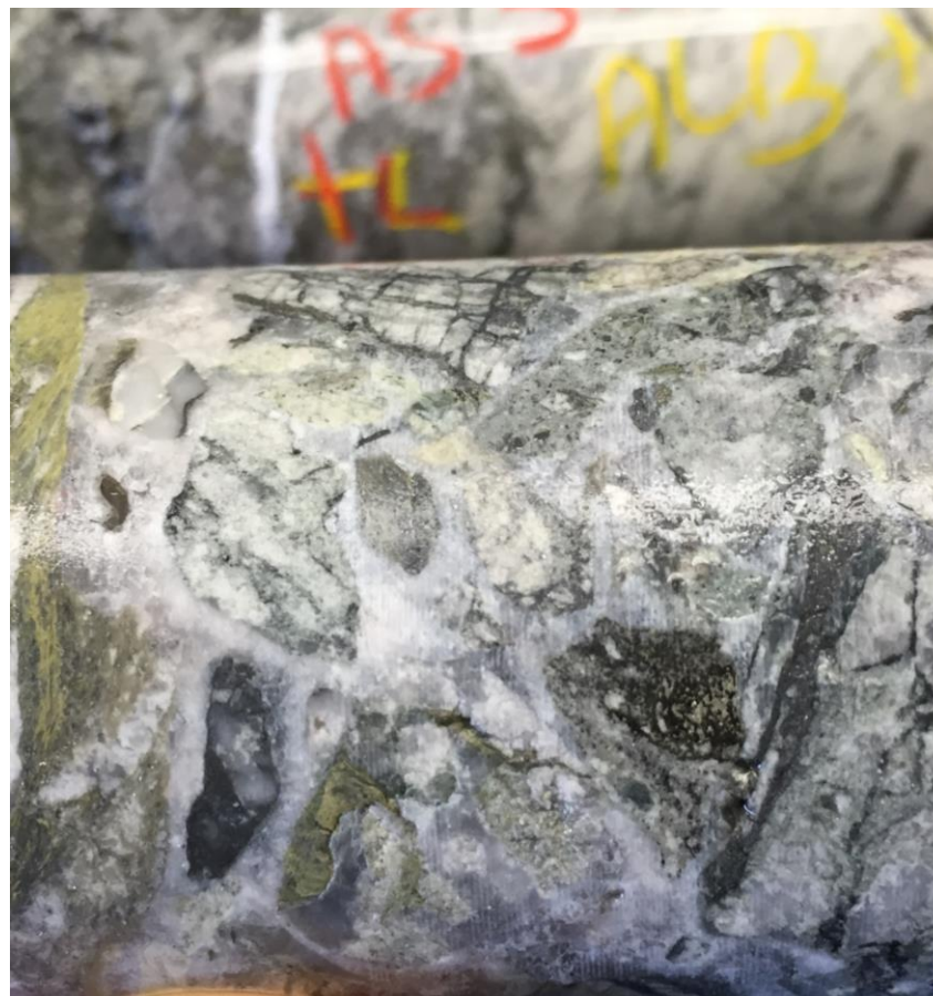
SAM-20-009 (AS ZONE) 373.60-374.45 (0.85m) Breccic interval with strong alteration in Alb-Sr. Moderate fuchsite and weak chlorite, tourmaline. AS: 0.5-5% in mm veinlets or disseminated PY: 0.5-1% along AB-QZ veins or disseminated
