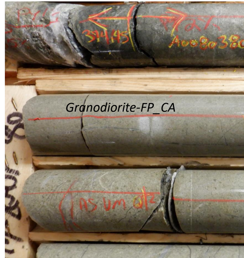
SAM-20-009 (AS ZONE) 374,45-382m (7,5m) 0.5-1% Pyrite, 0.3-1% arsenopyrite. AS is fine, aligned along Qz-Alb veinlets or and disseminated. 1% mm quartz veins
