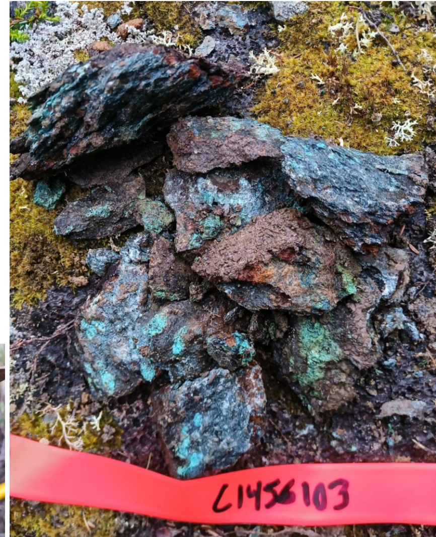
#C1456103: ultramafic ankerite schist, 15% malachite, 1% bornite in the schistosity
