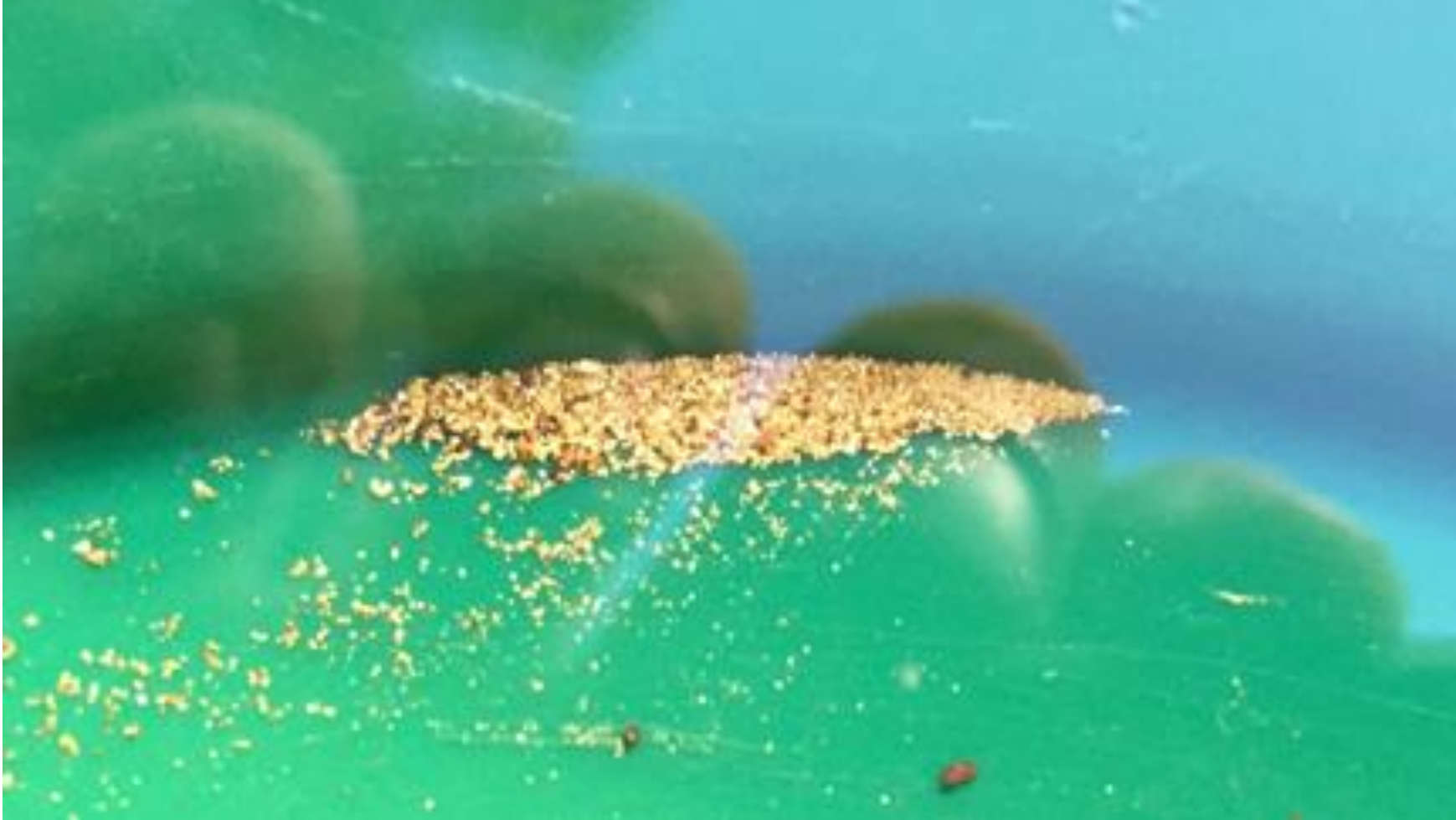
Figure 8. Free gold concentrated using a pan, extracted from gold-bearing soil developed on the iron formation. Winchester showing
