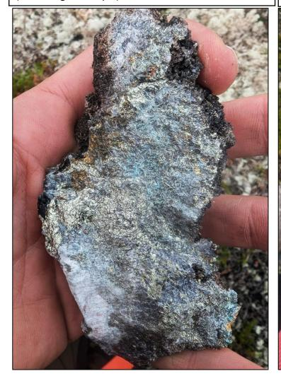
C1456560. Same dolomite boulder with intense tremolite calco-silicate alteration (skarn type) and pervasive mineralization of chalcopyrite-magnetite. **1.75% Cu** (selected grab sample)
