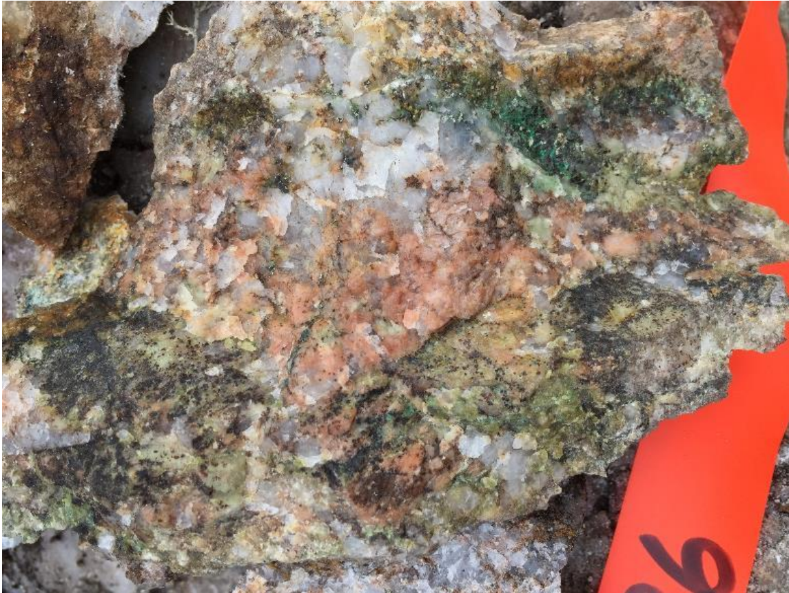
S410736 (outcrop) Granite, strongly altered in epidote, K-feldspar and injected with quartz, chlorite vein stockwork, disseminated chalcopyrite and pyrite 0.11 % Cu
