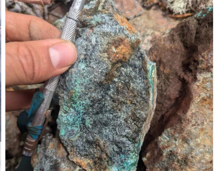
**C1456534 : 1,94% Cu, 143 ppm Co, 52 ppb Au, 18 ppm Mo**
