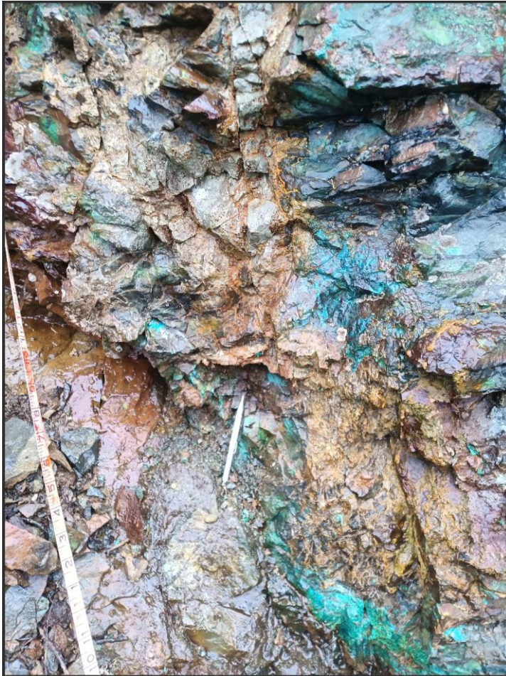
▲ #C1455753 : Mineralized veins or breccia containing massive chalcopryite and pyrite Pending results
