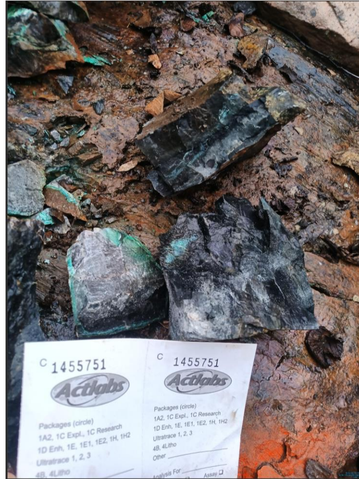
▲ #C1455751 : Cherty mudstone, mineralized with malachite (2 %) in halo and in the joints of the bedding. Pending results.
