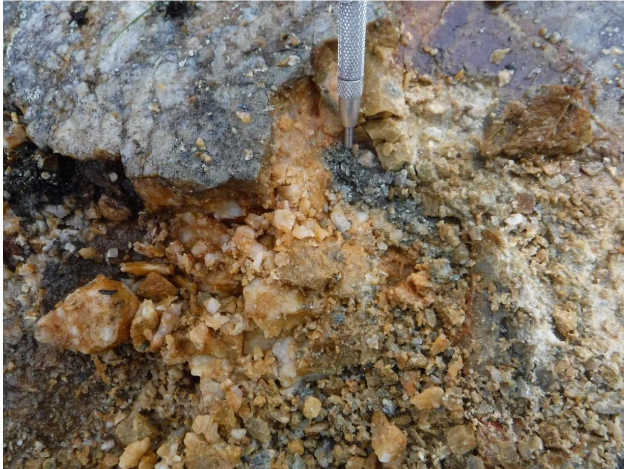
Quartz-Pyrite vein in quartzite outcrop 1.15 g/t Au (grab)
