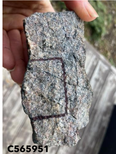
C565951 Altered alkaline rock (165 ppm Nb, 892 ppm Zr) with traces Py-Cpy
