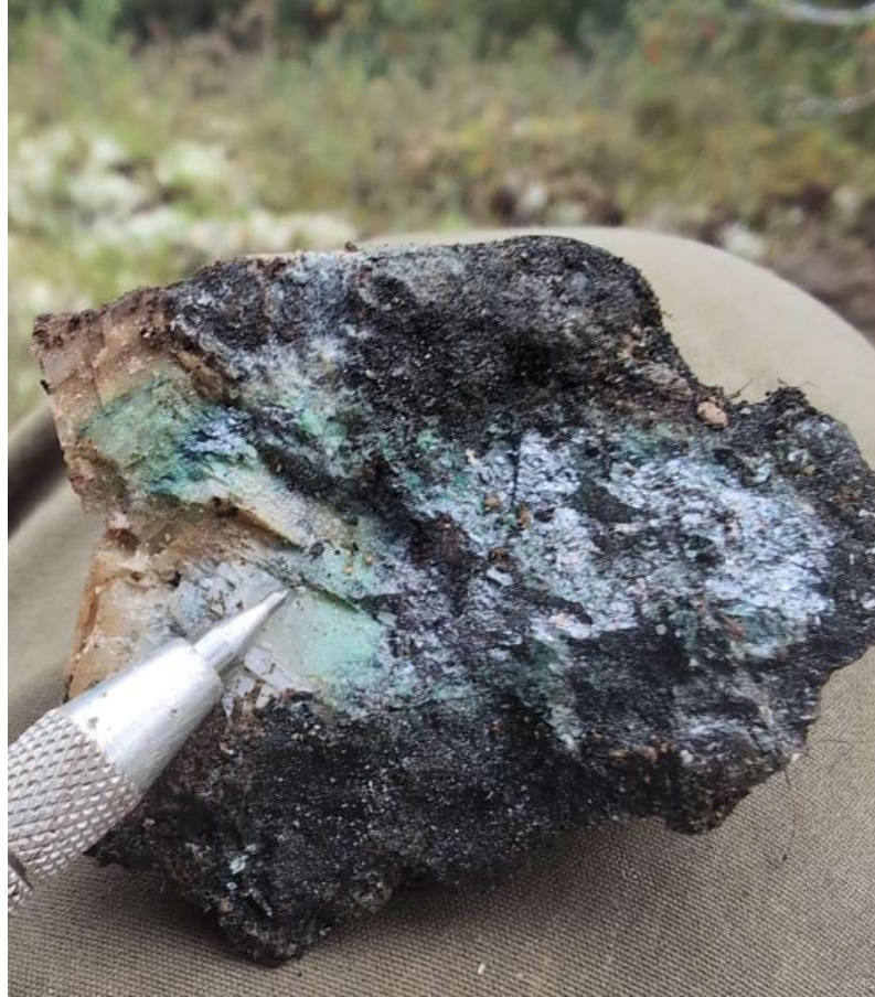
#C2130509 : 9.97% Cu, 2.40 g/t Au, 61.40 g/t Ag Centimeter-sized digenite cluster in a calcite vein
