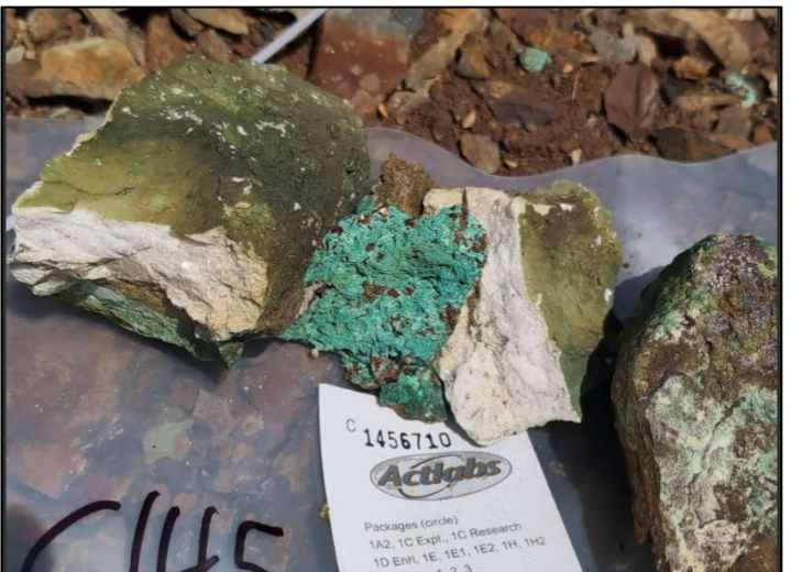
▲ #C1456710 : 12.30 % Cu, 0.36 g/t Au, 0.57 % REE, 0.02 % Co, 6.60 g/t Ag Calcite and malachite vein
