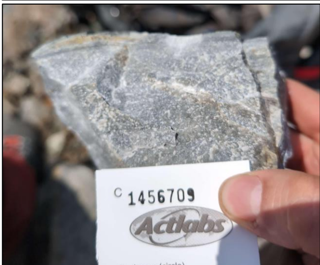
▲ #C1456709 : 0.39 % REE, 0.65 % Cu, 0.05 g/t Au, 0.008 % Co, 1.20 g/t Ag Mineralized siltstone with 3% chalcopyrite and highly carbonated
