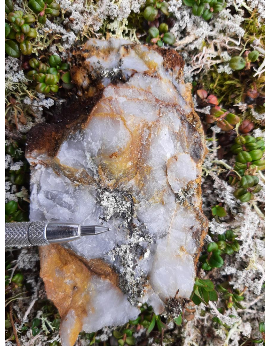
Quartz-Pyrite vein in quartzite outcrop 0.64 g/t Au (grab)
