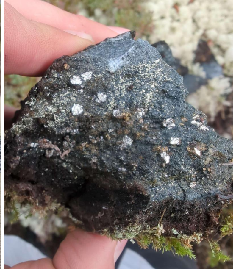
#C2130608 : 4.66% Cu, 0.20 g/t Au, 13.80 g/t Ag Pyrite and chalcopyrite mineralization disseminated in ultramafic rock
