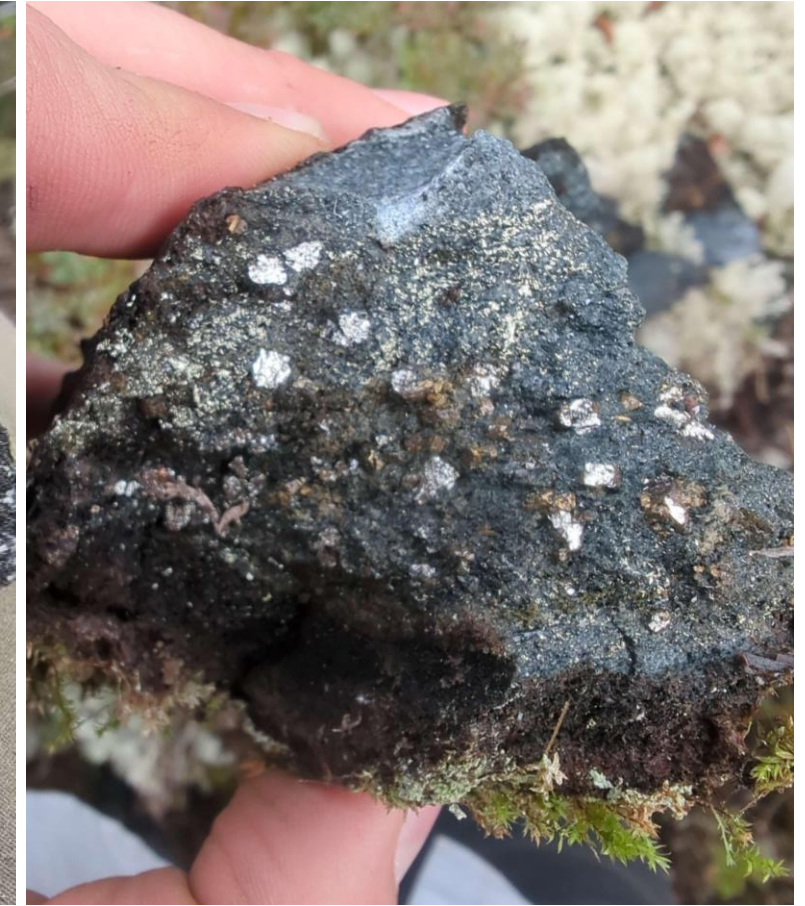
#C2130608 : 4.66% Cu, 0.20 g/t Au, 13.80 g/t Ag Pyrite and chalcopyrite mineralization disseminated in ultramafic rock
