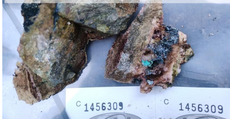
#C1456309: cm vein with specular hematite and malachite in an epidotized and albitized basalt
