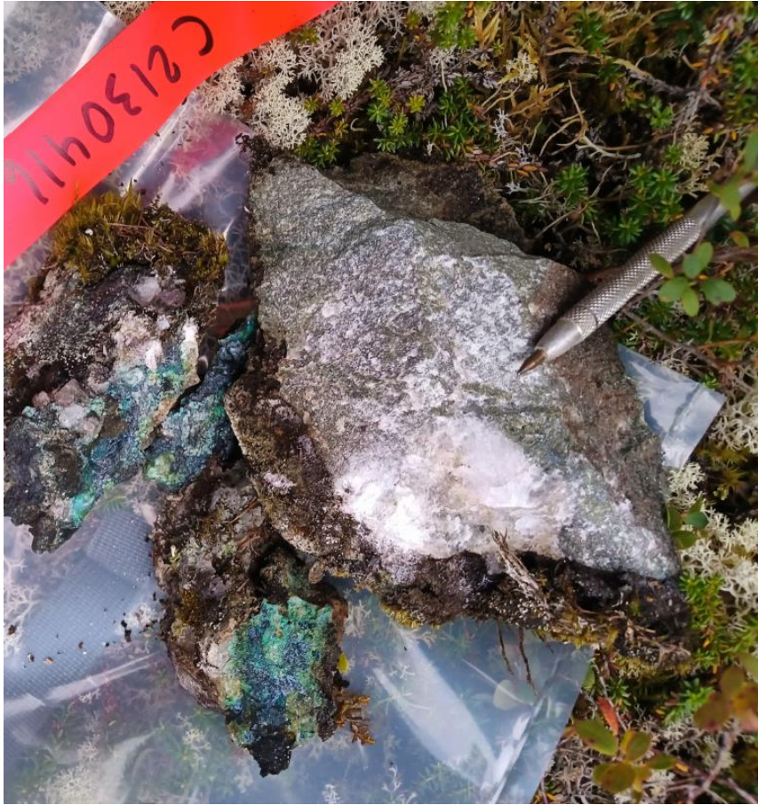
#C2130416 : 13.70% Cu, 4.83 g/t Au, 28.60 g/t Ag Clusters of digenite and malachite in a quartz and calcite vein within a mafic host rock heavily altered with epidote and albite
