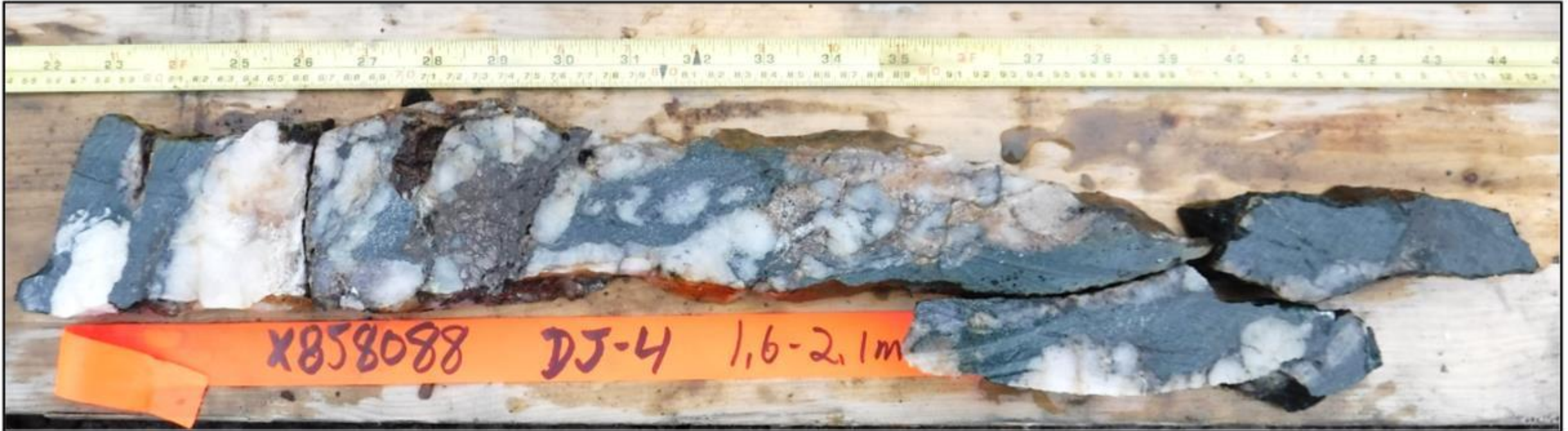
Figure 12: Example of the Didgeridoo mineralized zone, strongly altered in chlorite, small rusty quartz veins and pyrrhotite patches with traces of chalcopyrite. DJ-18-04 from 1.6 to 2.1m, X858088: 2.62 g/t Au.
