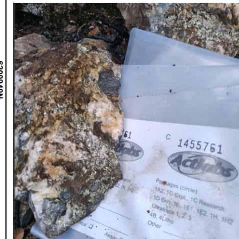
C1455761 : 6.12% Cu, 280 ppb Au, 1.77% REE, 675 ppm Co, 6.80 g/t Ag Shear-hosted calcite vein, 10% chalcopyrite, 2% malachite
