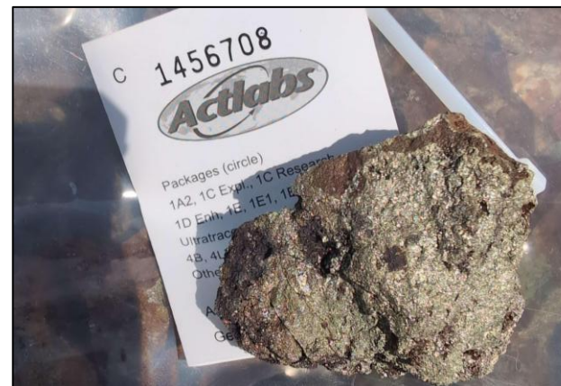
◀ #C1456708 : 31.60 % Cu, 6.92 g/t Au, 0.16 % REE, 0.20 % Co, 37.30 g/t Ag Chalcopyrite, malachite, azurite massive horizon
